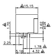
Electrical: 1.Voltage Rating:125 Vac Rms. 2.Current Rating:1.5 Amp. 3.Contact Resistance:40 Milliohms Max. 4.Insulation Resistance:1000 Megohms Min @500 Vdc. 5.Dielectric Strength:1000 Vac Rms 60Hz, 1Min. <u>Mechanical:</u> 1.Operating:750 Cycles Min. <u>Environmental:</u> 1.Storage:-40°C To +85°C. 2.Opertion:-20°C To +75°C.
