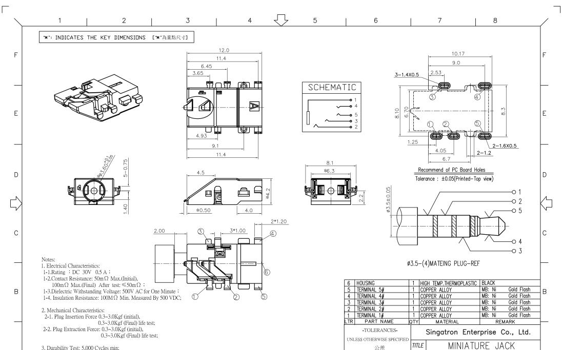
3. Durability Test: 5,000 Cycles min; 4. Operating temperature:  $-25^{\circ}C \sim +70^{\circ}C$ ; 5. Soldering Heat Resistance Reflow Soldering 260°C;
