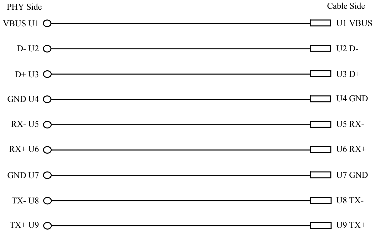
USB 3.1 GEN 1 Standard-A connector Pin Assignment
