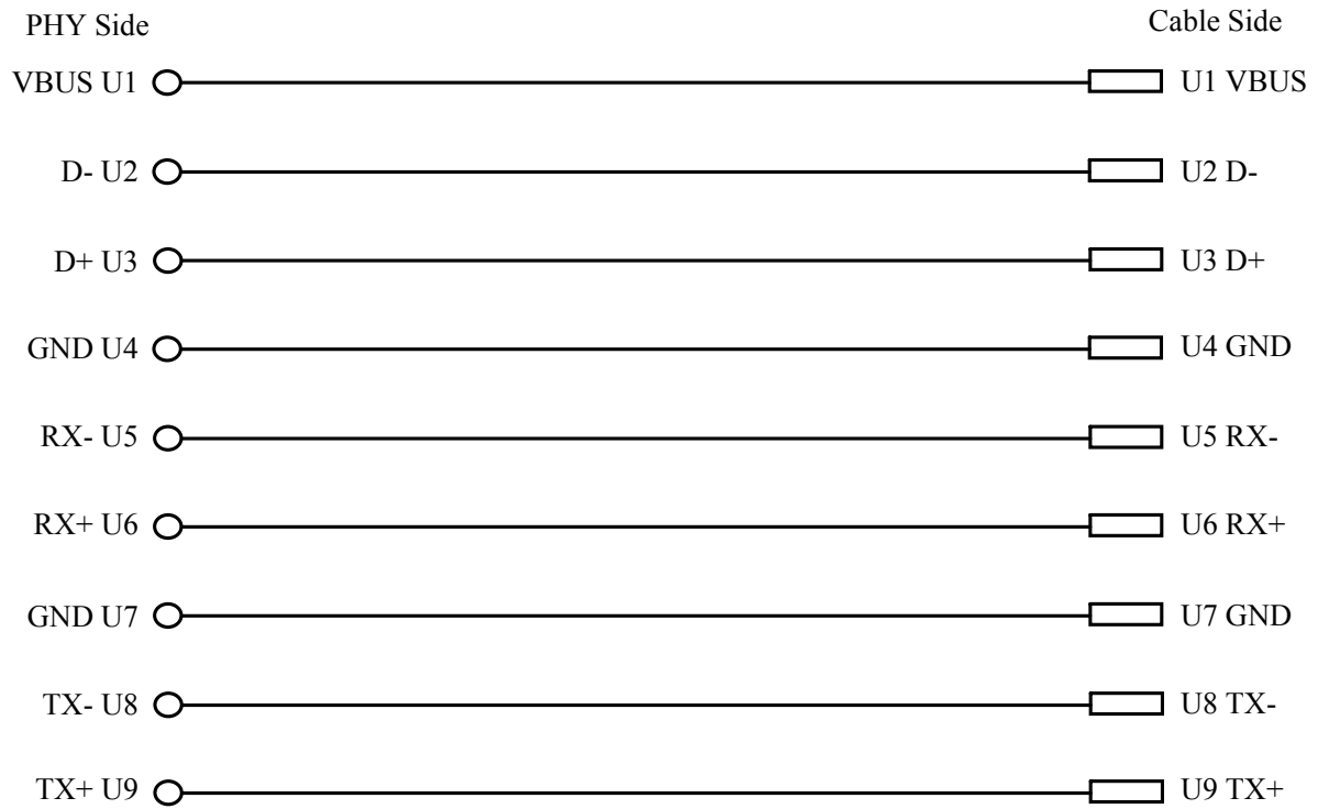
USB 3.1 GEN 2 Standard-A connector Pin Assignment
