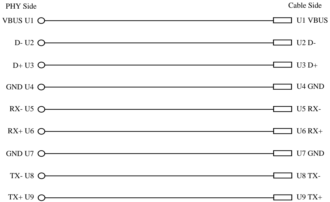
USB 3.1 GEN 1 Standard-A connector Pin Assignment
