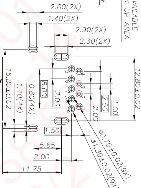
Recommended P.C.B Layout (THICKNESS=1.2mm)
